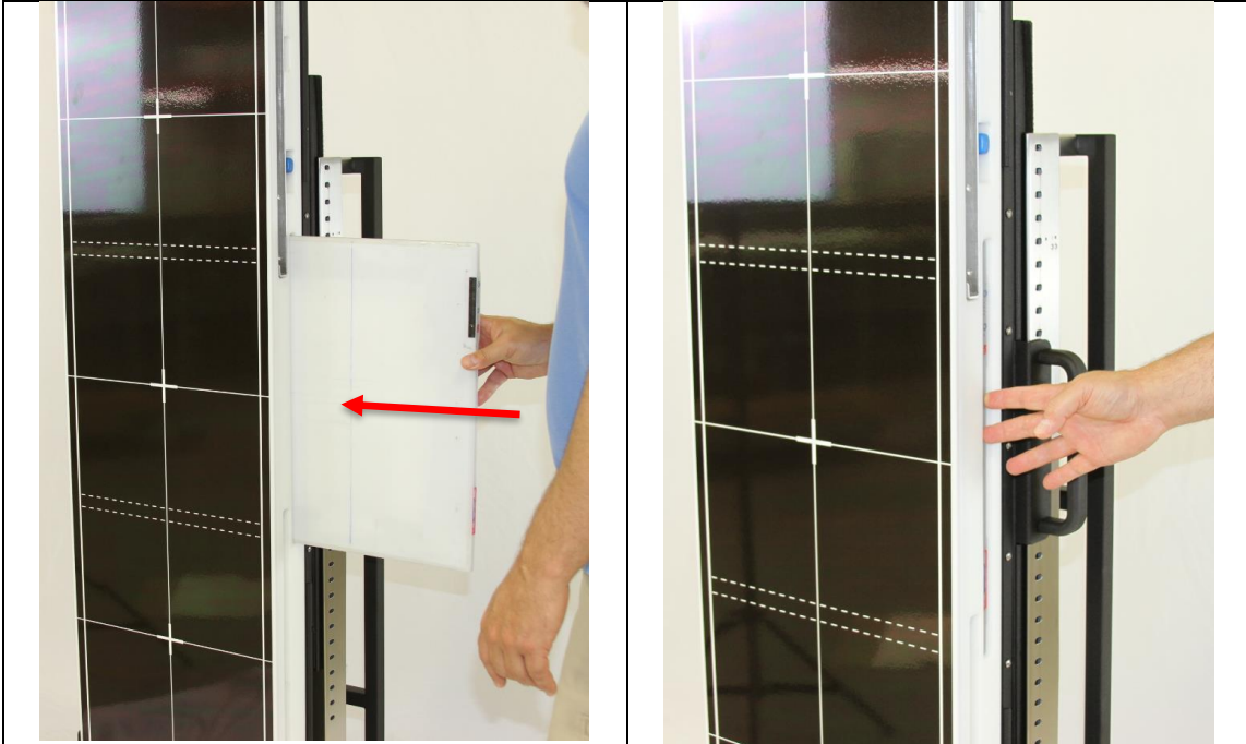
Mounting the DR Panels into the Bottom Detector Slots
