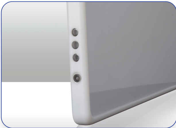
Cutouts for LEDs and PB
